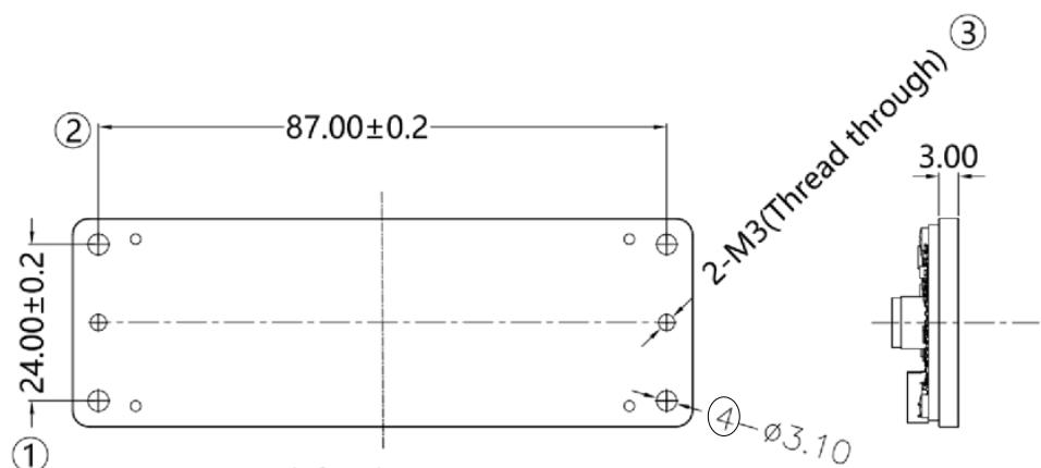
The depth origin X-Y coordinates are the X-Y centre of the left imager. The Depth module D421 origin reference from the left centre hole to the left imager centre is 18.5mm.
