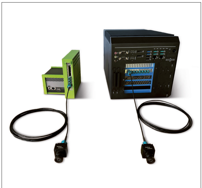
The SXVPU combines an AMD Kria™ SOM and FPGA fabric with a dedicated AI accelerator, delivering tens of TOPS of performance for neural network inference and high-throughput image processing.
